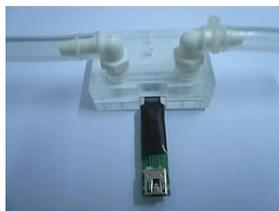
The sensor and flow cell combination is mounted on a platform (mote) which includes the sensor readout electronics, calibrant solution, fluidic control valves and wireless communication. These sensor motes have been placed at various important locations within the pilot plant.
